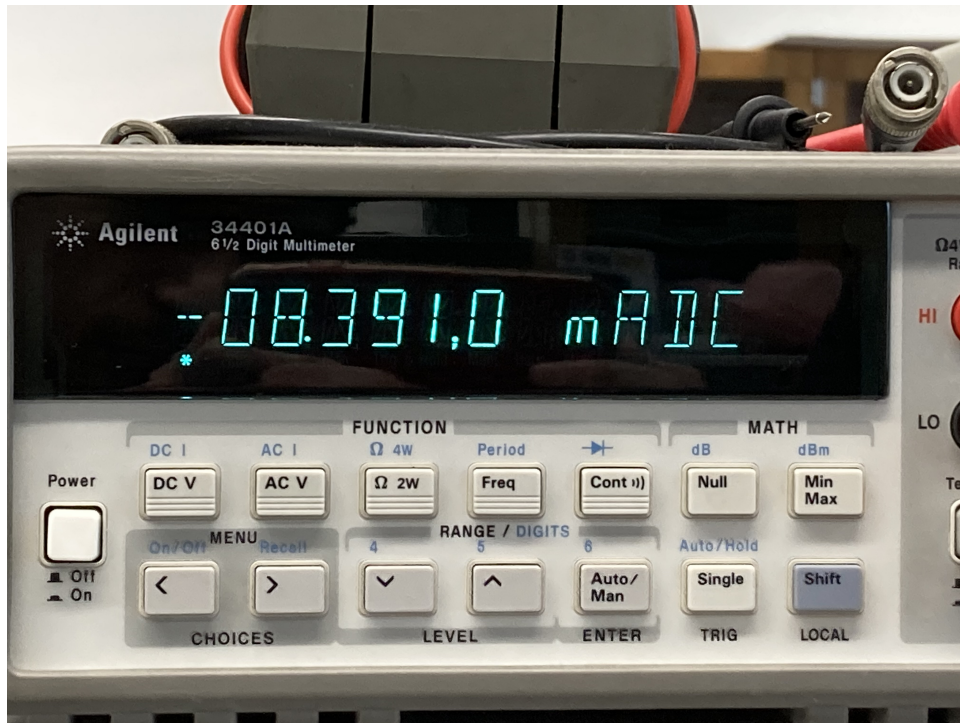
Figure 12: the current consumed by the 230 MHz oscillator with a 10 V supply; power use was then \sim 84 \text{ mW} .
